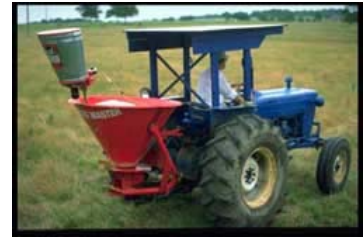
Herd GT77 seeder mounted on a fertilizer spreader.
