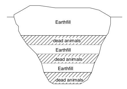
Typical for backhoe trench with 4-6 ft depth, at least 3 ft width, and variable length.
