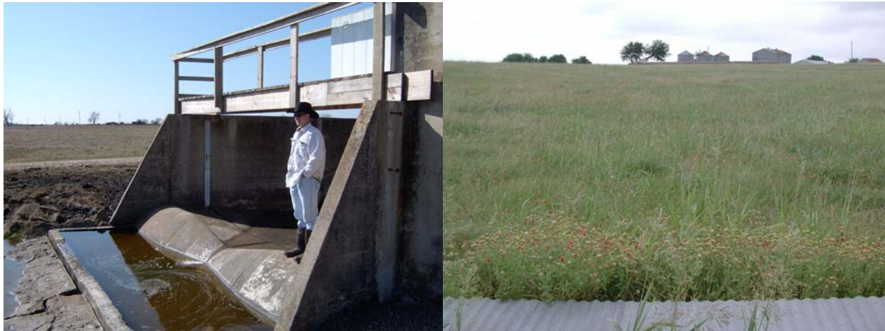
Figure 2. H-flume at site SW17 (left frame). Ungrazed native prairie at site SW12 (right frame).
