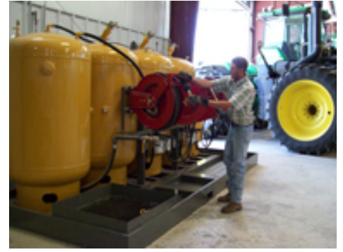
Figure 2: Portable tanks, nurse tanks, or skids (such as those provided by Sage Oil Vac, Inc. in Amarillo) are exempt from SPCC regulations and are not counted in the total on-site fuel and oil volume. Although secondary containment is not specifically required for this class of containers, take care to minimize the potential to drain fuel, oil, or waste oil into water sources. Any such discharge event is in violation of state and federal environmental laws.
