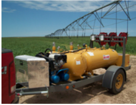
Figure 2: Portable tanks, nurse tanks, or skids (such as those provided by Sage Oil Vac, Inc. in Amarillo) are exempt from SPCC regulations and are not counted in the total on-site fuel and oil volume. Although secondary containment is not specifically required for this class of containers, take care to minimize the potential to drain fuel, oil, or waste oil into water sources. Any such discharge event is in violation of state and federal environmental laws.
