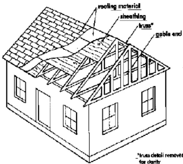
To inspect your roof's bracing, go into the attic. While working in your attic, you should wear clothing that covers your skin, work gloves, a hat, eye protection, and a dust mask. If your attic is not floored, be careful to walk only on the wood joists, or install boards wide enough to walk on as you work. Notice how the plywood is attached to the truss system. If most of the large nails or staples coming through the sheathing have missed the trusses,
